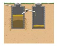
**Double leach-pit:** Two alternating partially lined (sealed on the bottom) pits, where one pit is used until it becomes full. At the same time, wastewater slowly permeates into the surrounding soil, which allows the easy removal of degraded, dewatered soil.
