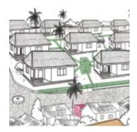
Small or simplified sewer network extended to public sewer **network:** Where appropriate, a network of smaller pipes might be useful for the collection and conveyance of wastewater to a public sewerage network.
