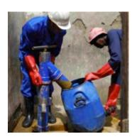
**Manual emptying:** The process of manually removing sludge from on-site sanitation solutions using human-power. Emptying can be done using buckets and shovels, or by using a portable, manually operated pump specially designed for sludge (e.g. "Gulper"). Sludge is then transported to a sludge treatment plant in containers using a pushcart or small 3-wheel transporter. Each trip can transport 350 litres.
