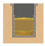
**Lined-pit:** A single or double hole lined with sand-cement rings, trapezoidal cement blocks or normal blocks, which might also be raised off the ground in areas with high water table or flood**prone.** Lined pits are more permanent and long lasting than unlined-pits, and preventing soil from collapsing. Sludge can be easily removed and the pit re-used many times (See Page 8).
